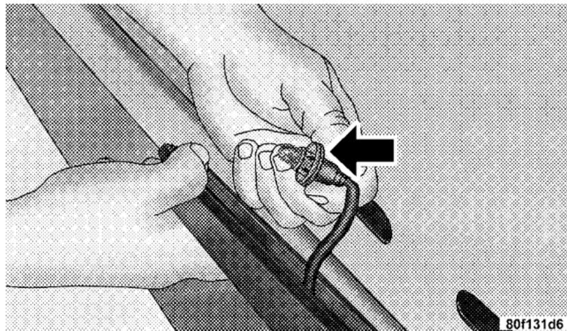
3. Pull bulb straight out from socket.
