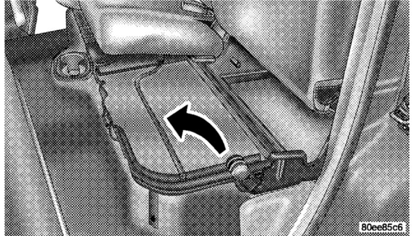
**Unfolding The Load Floor**
