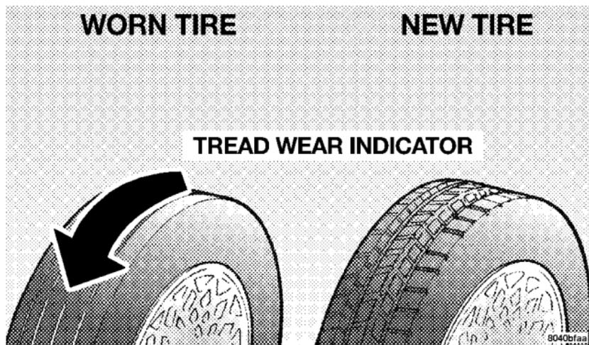
These indicators are molded into the bottom of the tread grooves. They will appear as bands when the tread depth
