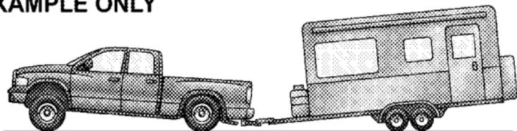
FIG. 1 WITHOUT WEIGHT DISTRIBUTION (INCORRECT)
