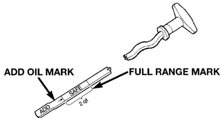
Never operate the engine with oil level below the “ADD” mark or above the upper “SAFE” mark.
