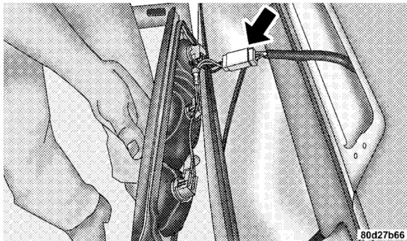
3. Turn desired bulb socket  $\frac{1}{4}$  turn and remove socket and bulb from housing.
